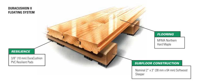
Slab Depression: 3/8" (10 mm) pad: 25/32" (20 mm) flooring - 2 5/8" (67 mm) • 33/32" (26 mm) flooring - 2 7/8" (73 mm) • 5/8" (16 mm) pad: 25/32" (20 mm) flooring - 2 7/8" (73 mm) • 33/32" (26 mm) flooring - 3 1/8" (79 mm)
