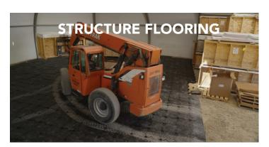
PortaFloor **MAX** was recently installed inside a Sprung® structure as a heavy duty reusable flooring system for inventory storage versus a gravel sub-base. The floor easily contoured to the structure's unique shape by including 6" wide cable-channeled **MAX** pieces that enabled a custom fit. **MAX** provided a firm stable surface for the rolling service doors. In structure installations, MAX can be installed inside the structure or extended beyond the sides for a clean and durable foundation.
