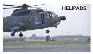
A HH3F Sikorsky (11,860 lbs./ 5,380 kg) Helicopter landed on PortaFloor **MAX** at a NATO training exercise in Italy. The 16,000 ft2/ 1,486 m2 site was installed by the Italian Air Force. **MAX** was secured at the perimeter and was used as a taxiway, landing and takeoff location for the HH3F. **MAX** was tested along side of the heavier counterpart, AM2 matting, as a viable option for a deployable landing facility.
