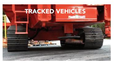
PortaFloor **MAX** was tested with a rotary blasthole drilling rig at a major high-technology Mining and Construction manufacturer. **MAX** was installed on a prepared sub base with **MAX** transition ramps for easy on an off access for the rig. Several maneuvers were performed by the 176,000 lbs / 79,832 kg drilling rig including; zero radius turning, raising the drilling mast and deploying the multiple jacks to raise and secure the rig.
