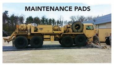
After a year of testing, the 416th Theater Engineer Command (USAR) has recognized the **MAX** flooring system as a deployable maintenance pad for their portable maintenance structures. Each area will be roughly 800 square feet and fit within a standard structure. The floor has been tested using the 54,900 pound M984 HEMTT Wrecker and light-weight aircraft aluminum plates to reinforce the point load weight of the jack stands.
