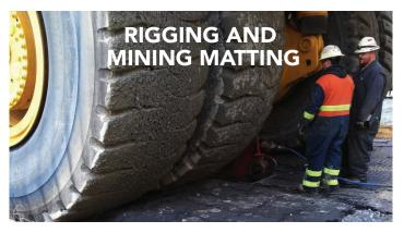
PortaFloor **MAX** was recently tested on site at a major mining pit as a re-locatable haul truck maintenance pad. The goal was to eliminate the need to pour a temporary concrete slab that needed to be removed in a few months. Three successful tests were completed. In the photo above, two tires of a Komatsu 930e were lifted on **MAX** using an 18" diameter pneumatic jack. The back axles of the truck were also lifted on **MAX**, using a B & D Super Jack.
